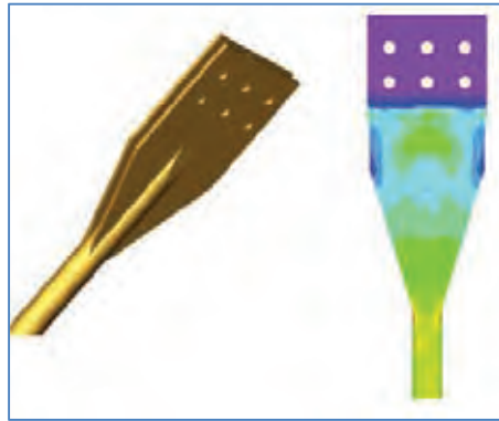
Figure 9. Fatigue assessment based on geometric stress ranges.
