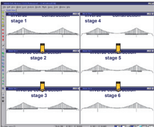
Display of Inverse Construction Stage Analysis models reflecting members, boundary conditions and loadings pertaining to each stage
